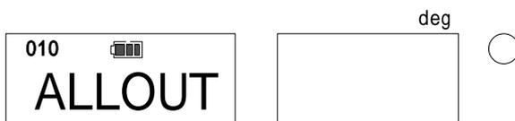
Press MD to set all data output display (above), and press MEM to process all data output. (Press C key to returns to measuring condition).
