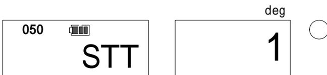
Use **MEM** key to set the lower limit of the output data range. Press **MD** to confirm the lower limit and the display shows the number data to transfer (Press **C** key to cancel).
