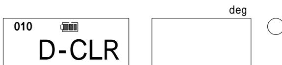
Press MD key to set 1 work data deletion (above), and press MD key and C key at the same time to process deleting.
