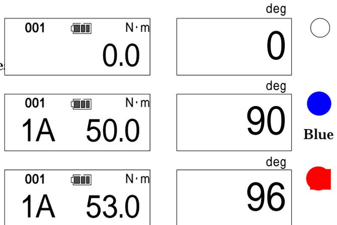
Upon reaching the set angle, the buzzer goes off and the blue LED turns on.
