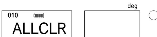
Press MD key to set all data deletion (above). (Press C key to returns to measuring condition). Press MD key and C key at the same to process deleting.
