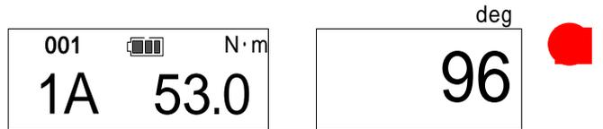
If the tightened angle exceeds the upper limit, another buzzer goes off and the red LED starts to blink.
