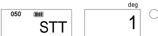
Use **MD** key to show the lower limit of the data range to delete, and press **MD**. The Display shows the number of data to delete (Press **C** to cancel).
