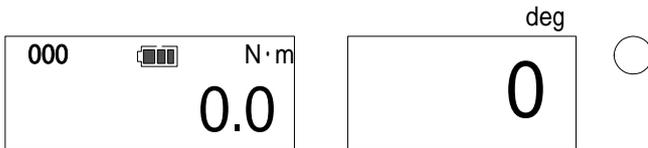
Press MD key for more than 2 sec. After the display changes to tightening mode setting, release the key.
