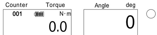
Upon reaching the snug torque, the buzzer goes off for 0.5 seconds and the angle measurement starts. When it reaches 20 degrees before the set angle, the buzzer starts to sound on and off continuously (the buzzer will not sound if the set angle is below 20 degrees).
