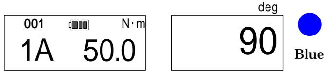
Buzzer starts to sound when it reaches 20 degrees from the set angle.
