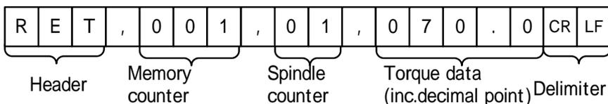
**Output image sample of production tightening mode**
