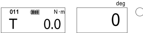
In PEAK mode, press MD key, then it turns to 1 work data output display (below).
