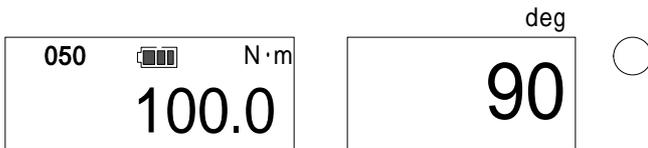
Press **MD** key to confirm the upper limit, then the display proceed to the lower limit setting.
