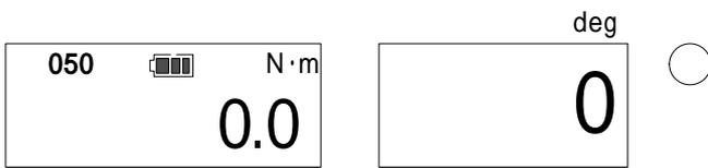
Press  key to reverse the memory counter to check the previous measured data.
