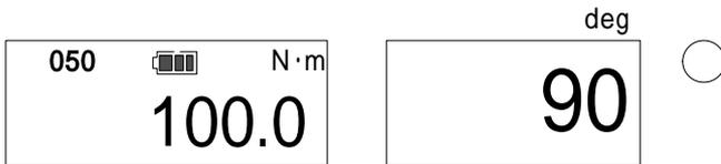
Press **MD** to confirm the upper limit, then the display proceed to the lower limit setting.
