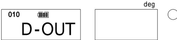
Press MEM key to process the data output of the last tightened work.
