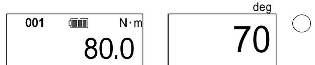
Upon reaching the set tightening angle, the buzzer goes off and the blue LED turns on.
