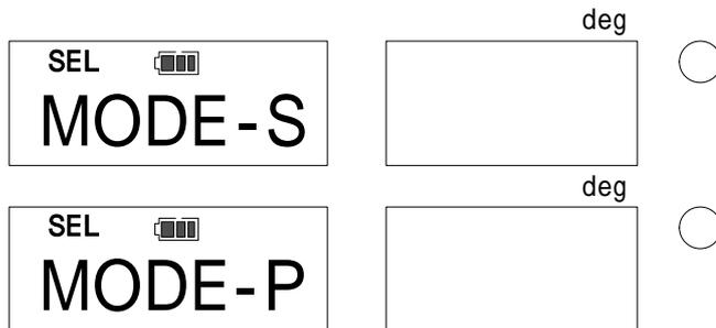
Single Spindle Tightening: Set the snug torque and tightening angle to conduct the angle method tightening from the snug torque to the set angle (1 spindle only)
