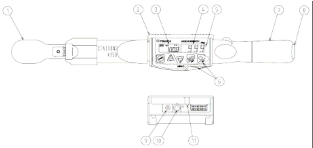
Interchangeable head: QH is packaged as standard accessory. Other TOHNICHI interchangeable heads are also applicable (SH, SH-N, RH, QH, RQH, DH, HH, FH).
