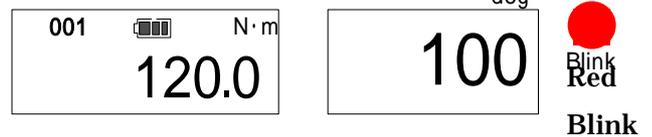
After releasing loading, press MEM key to make judgment to see whether the tightened torque/angle is within set range (The judgment is conducted automatically when auto memory/reset is set).
