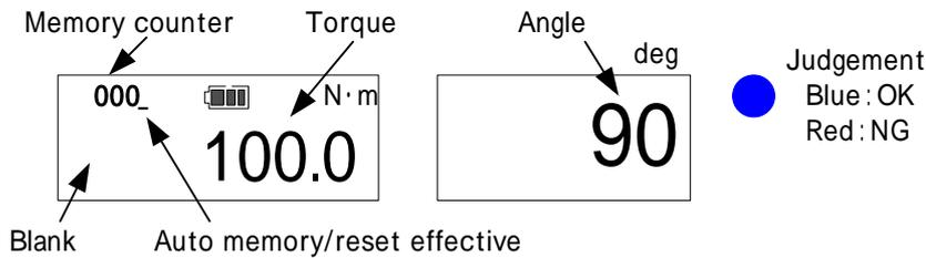
Press the reset switch or unplug the discharge plug to reset and it starts in RUN mode.
