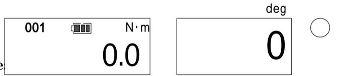
Upon reaching the set angle, the buzzer goes off and the blue LED turns on.
