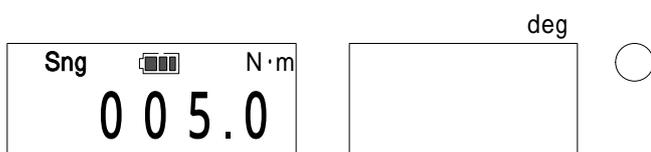
Use  key to select the digit, and change values with  key. Press MEM key to confirm and proceed to the next (Press MD key to proceed without saving. Press C key to return to RUN measuring mode).
