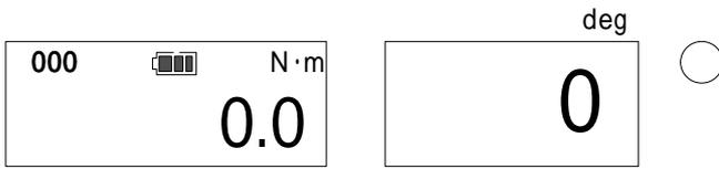
In RUN mode (check the counter shows 000), press MD key for more than 2 sec. After the display changes to tightening mode setting, release the key.
