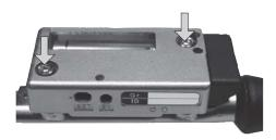
(5) Attach the battery cover and tighten the 2 screws with the torque driver. (Tightening torque:  $T=63cN\cdot m$ )
