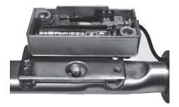
(2) Lift up the antenna connector and pull it out. (Cut the antenna with nippers or a similar tool.)
