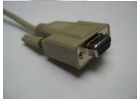
RS232C cable Please use D-sub9 pin female RS232C straight cable which is on the market.
