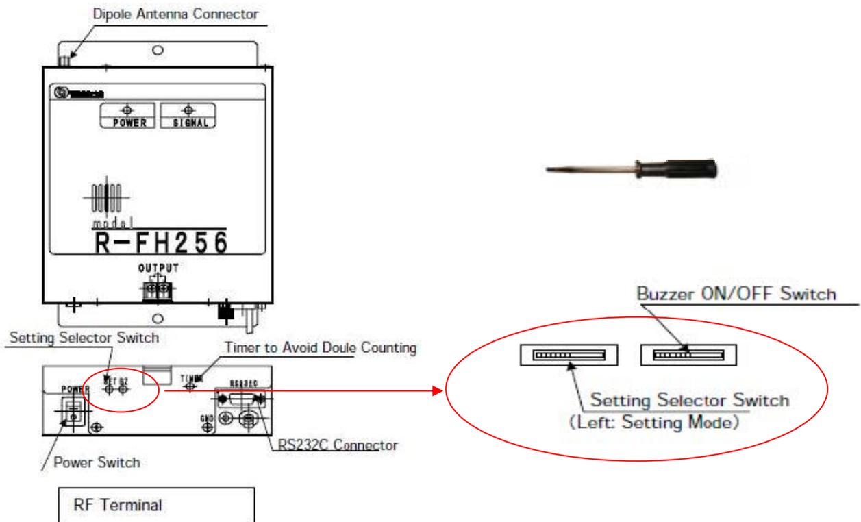
Slide the "Setting mode switch" to the left by using small flathead driver.
