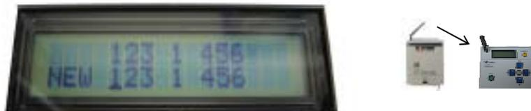
After the channel number has been set press "get switch" again to confirm the receiver's channel number has changed to the new frequency.
