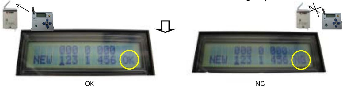
After the channel is selected press "Set switch". When the receiver gets the new channel number "OK" will be displayed,
