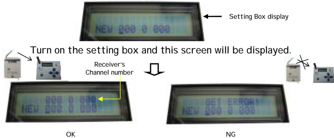
Press "Get button" and Receiver's channel will be displayed on the first line.
