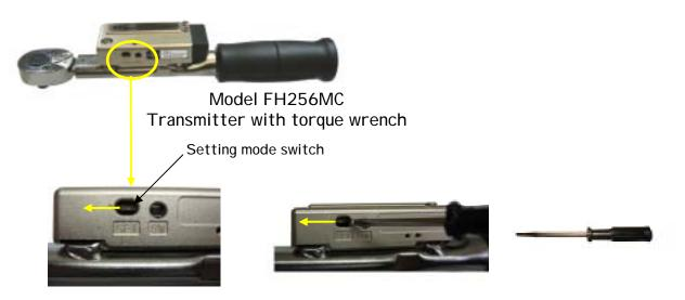
Slide the "Setting mode switch" to the left by using small flathead driver.
