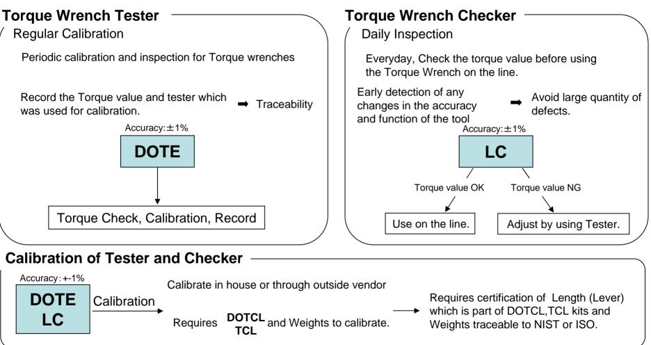
The calibration period is dependent on internal quality management accuracy requirements and/or frequency of use.
