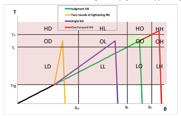
Trg: Trigger torque, TL: Lower limit torque, TH: Higher limit torque,
