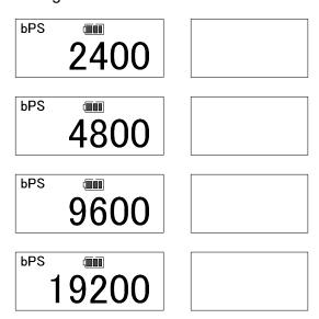
Select the baud rate using upper or down arrow keys. Press "MEM" key to save setting and go to next. Press "MD" key to skip setting and go to next. Press "C" key to go back to RUN mode (measurement mode).
