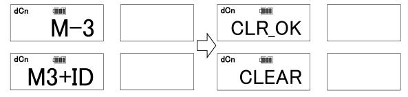
When change the communication format setting the measured data would be cleared.
