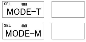
When set to "MODE-M" the double tightening detection angle setting will be skipped. If there is double tightening detection angle setting and change to "MODE-M" the double tightening detection angle will be set to "0".
