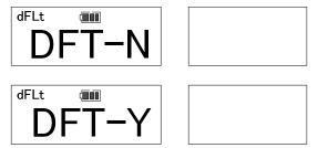
Select the "DFT-Y" or "DFT-N" using upper or down arrow keys. When display shows "DFT-Y" and press "MEM" key, the tool is factory reset. to save setting and go to next. Press "MEM" key on "DFT-N" or press "MD" key to skip setting and go to next. Press "C" key to go back to RUN mode (measurement mode).
