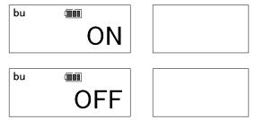
Select the buzzed is turned ON or OFF using upper or down arrow keys. Press "MEM" key to save setting and go to next. Press "MD" key to skip setting and go to next. Press "C" key to go back to RUN mode (measurement mode).
