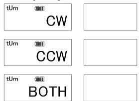
Select the direction using upper or down arrow keys. Press "MEM" key to save setting and go to next. Press "MD" key to skip setting and go to next. Press "C" key to go back to RUN mode (measurement mode).
