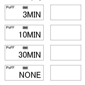
Select the timer using upper or down arrow keys. Press "MEM" key to save setting and go to next. Press "MD" key to skip setting and go to next. Press "C" key to go back to RUN mode (measurement mode).
