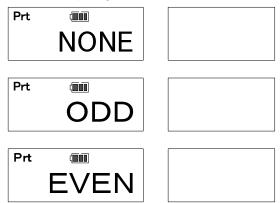
Select the parity using upper or down arrow keys. Press "MEM" key to save setting and go to next. Press "MD" key to skip setting and go to next. Press "C" key to go back to RUN mode (measurement mode).
