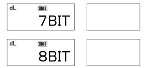
Select the data length upper or down arrow keys. Press "MEM" key to save setting and go to next. Press "MD" key to skip setting and go to next. Press "C" key to go back to RUN mode (measurement mode).
