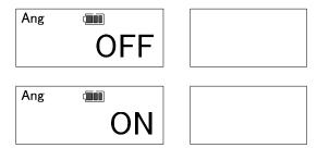
Select angle feature is ON or OFF using upper or down arrow keys. Press "MEM" key to save setting and go to next. Press "MD" key to skip setting and go to next. Press "C" key to go back to RUN mode (measurement mode).
